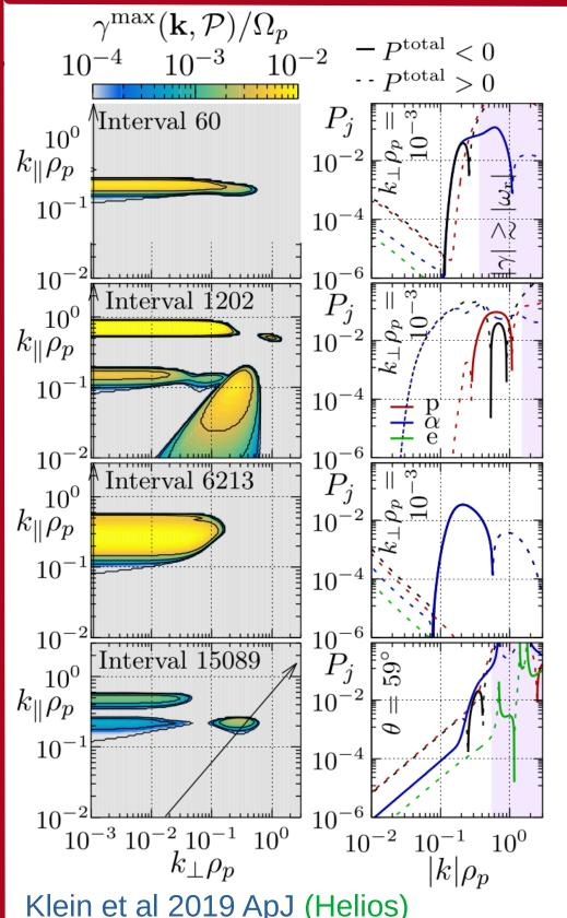
Using Nyquist's criterion enables the study of instability properties across a wide range of VDF parameters and wavevectors, and will identify when several different instabilities can be driven by different sources of free energy (e.g. by both the proton anisotropy and relative alpha drift, fourth row) **or** when a secondary population acts to reduce the growth rate of an unstable mode (e.g. second row).
