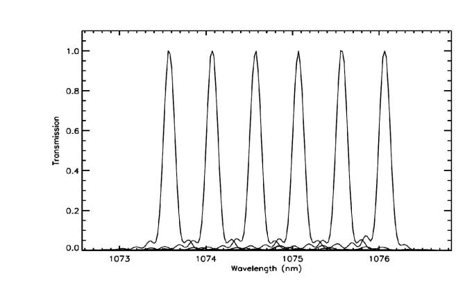
An example of 6 tunings of the filter in the vicinity of the Fe XIII 1074.7 nm line is shown here.
