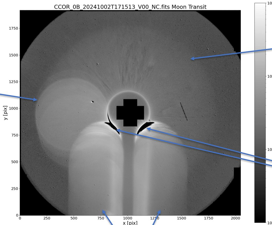
Default on the occulter (was observed during ground testing)
