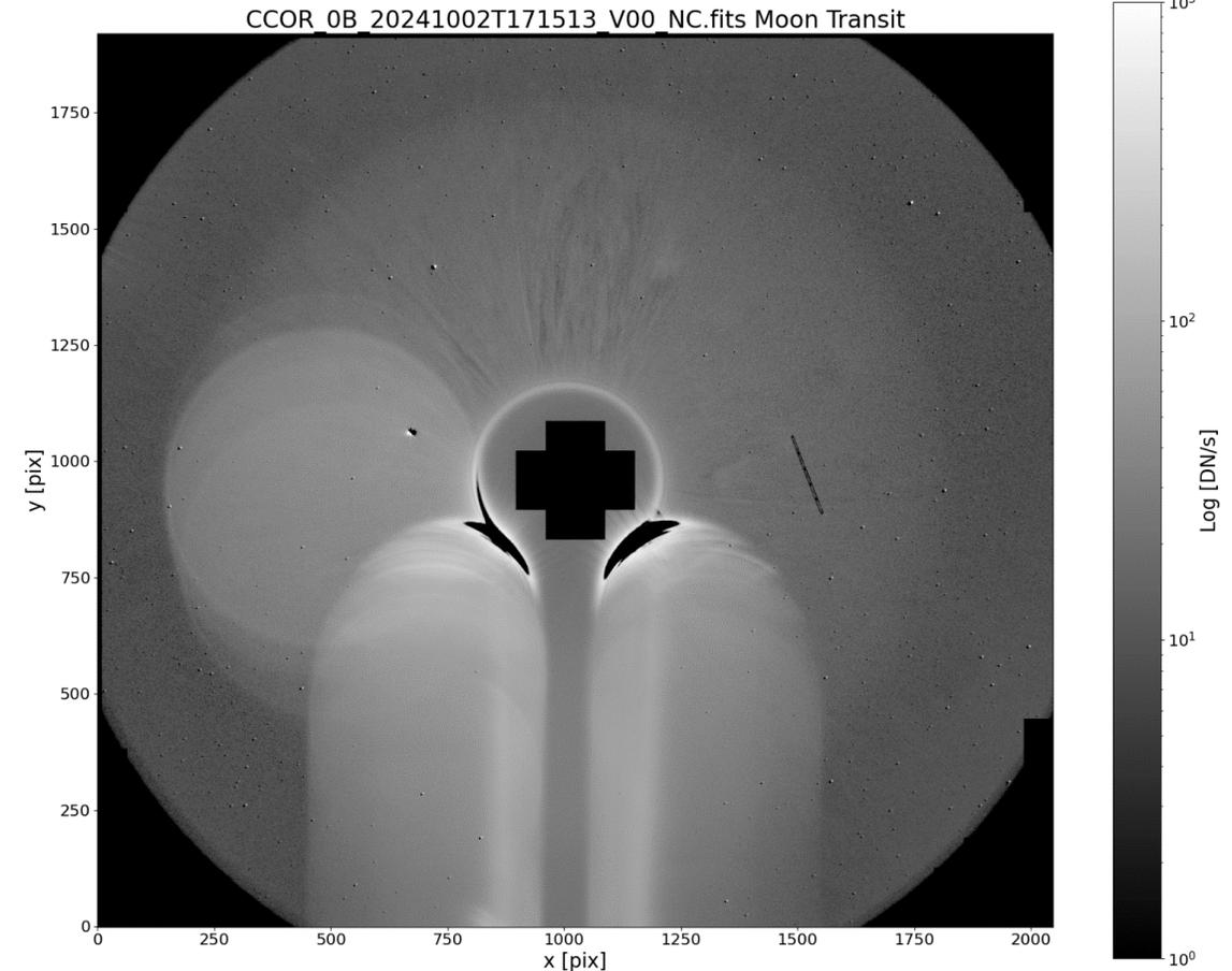
Straight difference between post-eclipse (18:00 UT) and eclipse image. Need additional post processing but all the expected stray-light features are present.
